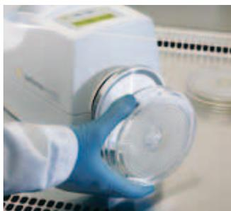
A new developed system for sampling airborne organisms that allows impaction onto culture media plates, where the plates function directly as collection heads. This means that the collection properties are integrated right into the culture media plates. Metal sieve plates or metal collection heads with slots, which have to be sterilized for routine samplings on a regular basis, are eliminated. Now, non-sterile sieves or slots have become a thing of the past.
