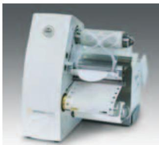
Fully automated membrane filter dispenser for individually sterile cellulose nitrate filter discs.
