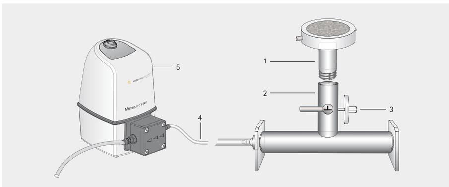
The filter station is directly connected to a vacuum fluid pump for simultaneous transfer of the filtrate to waste.
