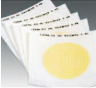
In the standard membrane filter method, a membrane filter with the appropriate pore size is placed in a filter holder and the sample is filtered. Any microorganisms present in the sample are retained by the pore structure on the surface of the membrane filter. The membrane filter is then placed on an appropriate culture medium and incubated to detect these microbes.
