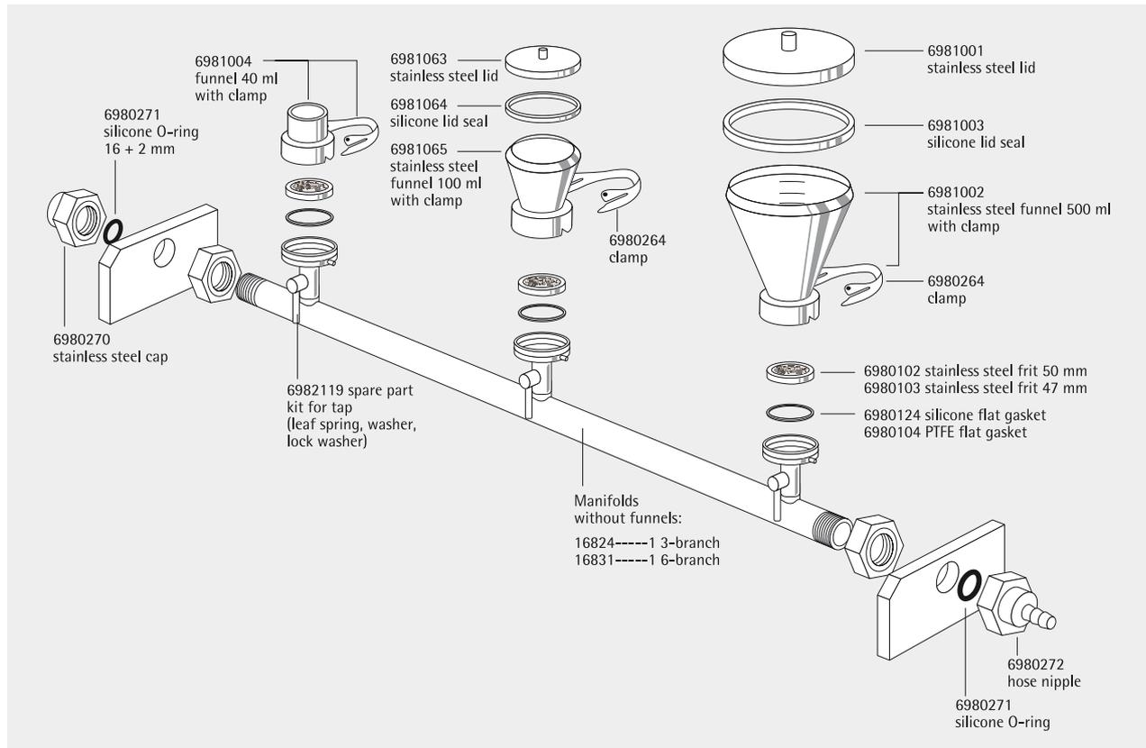
**Individual stainless steel filter holders, pre-assembled with stainless steel funnels and lids**
