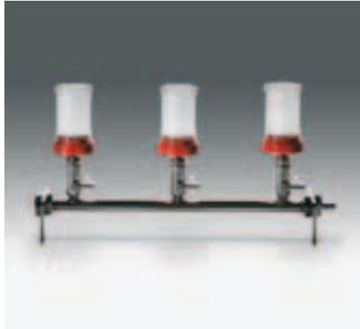
The low height of the manifold ports is particularly advantageous for working on a clean bench. For low number of samples, we recommend the use of the 1-branch manifold 16844 or the individual base 16841 on the top of a suction flask. For large number of samples, we recommend the 3- or 6-branch manifolds.
