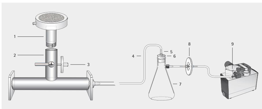
The filter station is connected to a suction flask, which is connected to a filtrate-protected vacuum pump.
