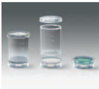
The membrane filtration method is the suitable technique for microbiological analysis of pharmaceuticals, water, cosmetics, foods and beverages. The use of ready-to-use disposable units is optimal for these applications.
